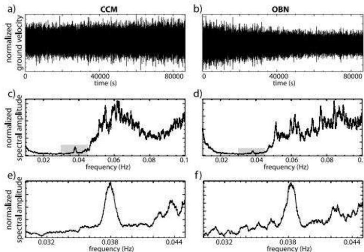
**Figure 1.** Examples of observation of the 26 sec (0.038 Hz) microseism from analysis of day-long vertical component records of seismic noise at stations CCM and OBN during August 22, 2004. Station locations are shown in Figure 3a. (a, b) Seismograms. (c, d) Amplitudes of the Fourier spectra. (e, f) Spectra zoomed around the 26 sec peak (indicated with gray boxes in Figures 1c and 1d).
